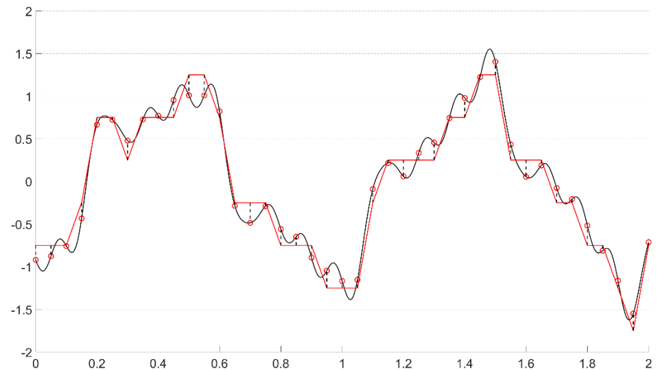
Figure 5: A signal sampled at 20 Hz. Discrete-time sampling (left panel) allows for continuous y-axis ( \mu\text{V} ) values, whereas digitally-sampled signals (right panel) must use a limited number of y-axis values. The three bit converter illustrated here (right panel) allows for 2^3=8 distinct values, providing only a coarse approximation of the signal voltage. The right panel depicts the discrete sample value (red circle) and the 3-bit digital equivalent (red line), and the discrepancy (dashed vertical black lines).
