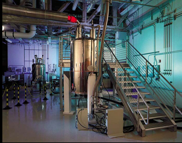
National laboratory's high magnetic field (18.8T) NMR spectrometer.
