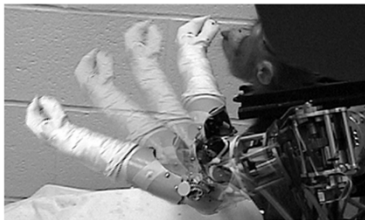
Fig. 4. A monkey is feeding himself with the aids of a robotic arm by producing the same pattern of neural activity in the motor cortex as would be required to move his own limb. The trajectory of the robot arm is depicted sequentially. In expectancy of the piece of an apple, the monkey protrudes his tongue. From the monkey only the head is visible. (We thank Dr. Andrew Schwartz, from the School of Medicine, University of Pittsburgh, Pittsburgh, USA, for this picture and for the permission of reproduction.)
